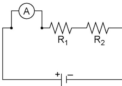
3. Remove the ammeter, reconnect the circuit, and then break the circuit between  $R_1$  and  $R_2$ . Measure the current through this point. Record this value as the current going into  $R_2$ . (Don't forget the units!)
