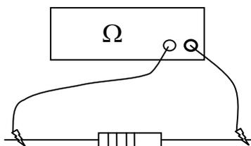
Figure 1. Measuring the resistance of a resistor.
