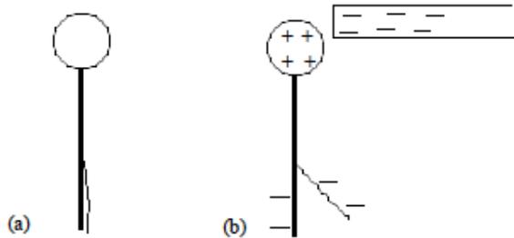
(a) If the electroscope is neutral and no charges are nearby, the leaves will hang straight down. (b) A charged rod near the plate causes the leaves to rise.
