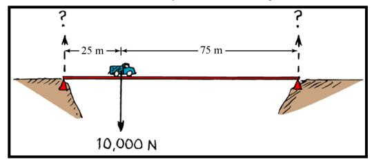
a. What torque does the weight of the truck exert about the support at the right end of the bridge?
